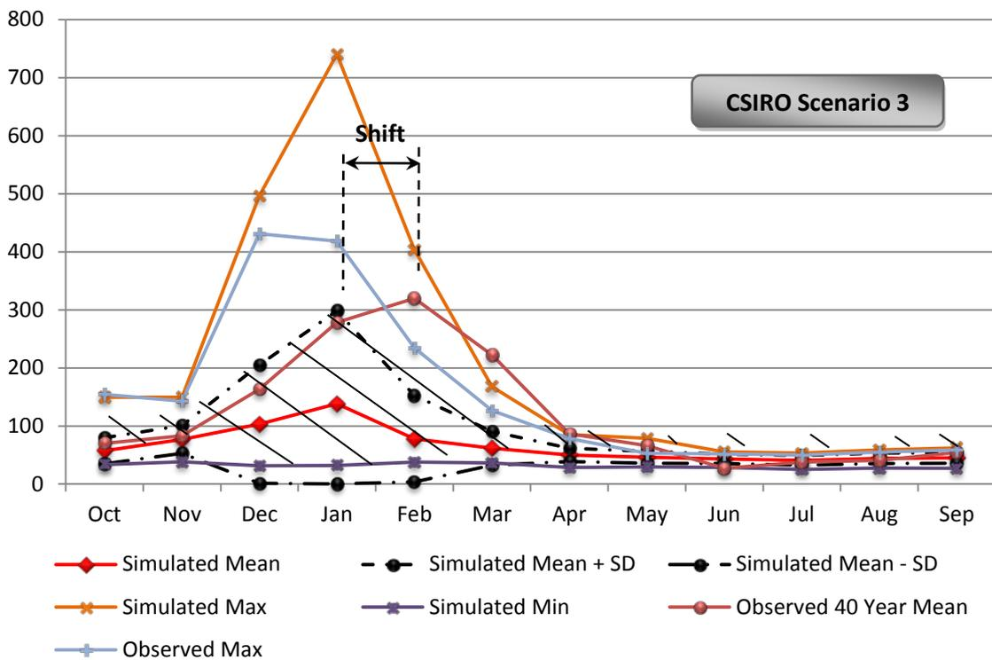
**Figure 6.46: Simulated Mean, Maximum, Minimum, One Standard Deviation under CSIRO and Historical Mean and Maximum Monthly Stream Flows**
