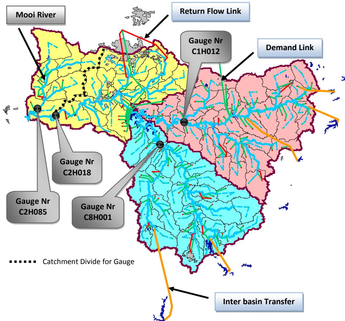
Figure 5.18: Schematic of Present Day Setup of the UVRB in WEAP
