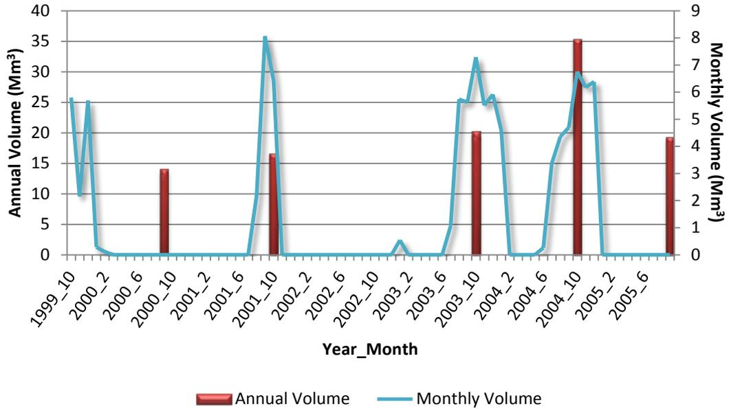
**Figure 5.6: Annual & Monthly Volume of Water Transfer for Zaaihoek - Grootdraai System**
