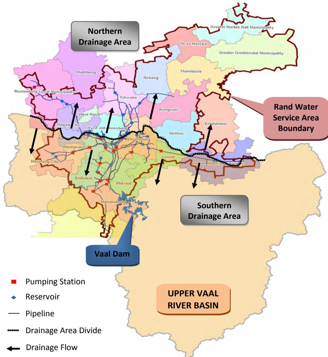
**Figure 5.8: Service Area of Rand Water and its Drainage Divide**
