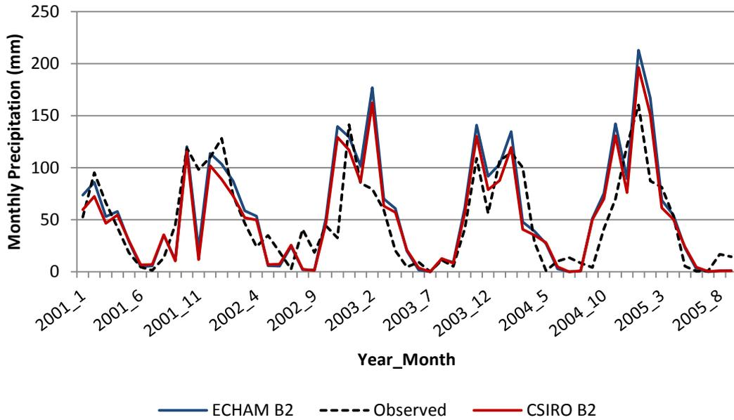
Figure 6.3: Time Series Plot of Observed against ECHAM4/ CSIRO B2 Precipitation
