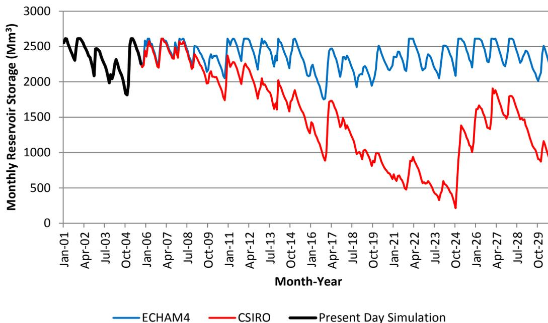
Figure 6.37: Vaal Dam Simulated Monthly Reservoir Storage under Scenario 2
