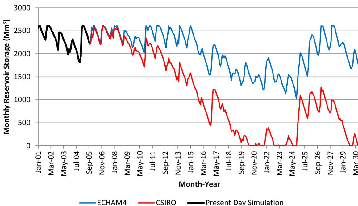
Figure 6.27: Vaal Dam Simulated Monthly Reservoir Storage under Scenario 1
