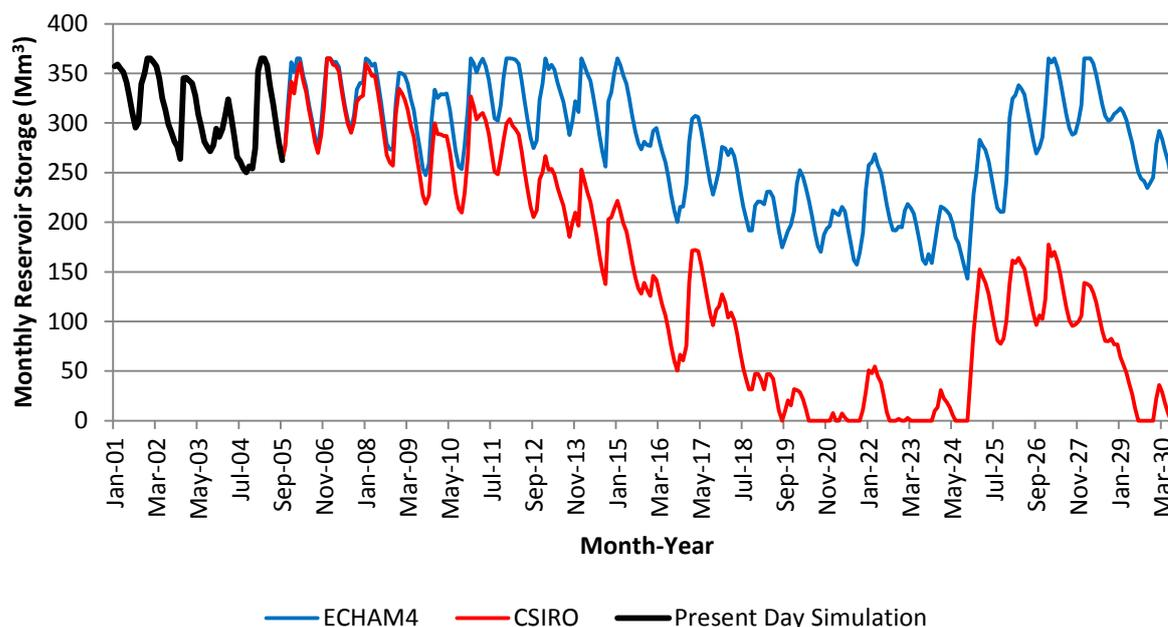
**Figure 6.28: Grootdraai Dam Simulated Monthly Reservoir Storage under Scenario 1**
