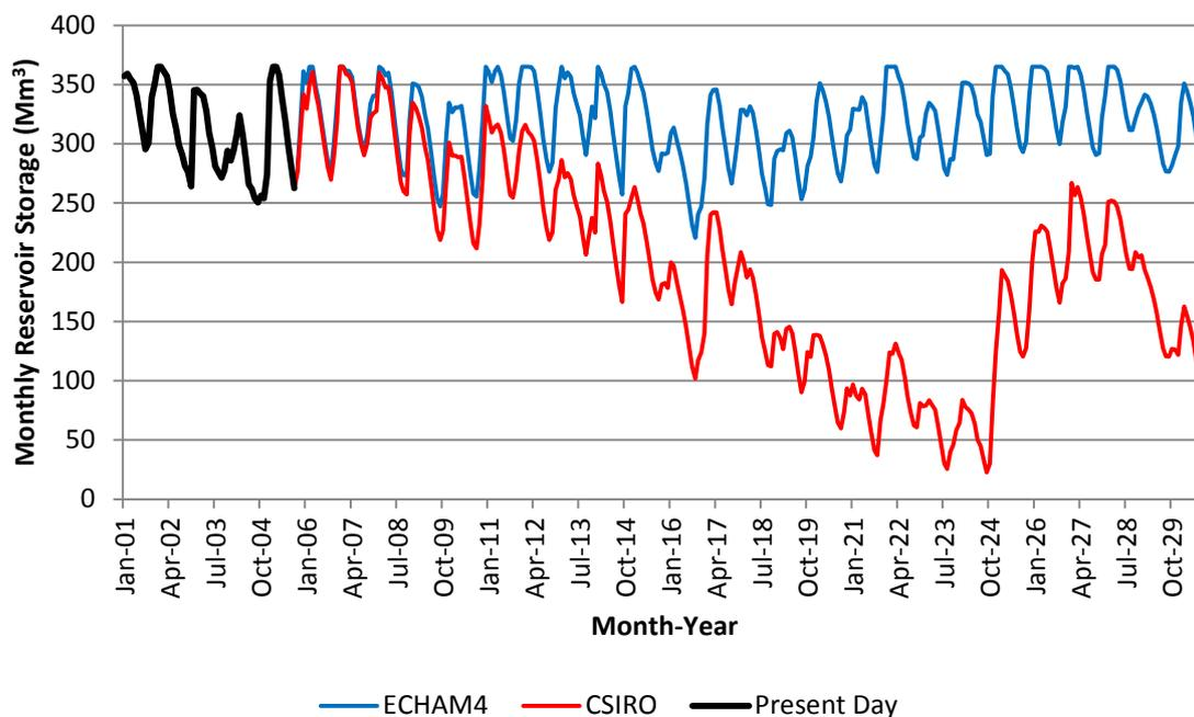
Figure 6.38: Grootdraai Dam Simulated Monthly Reservoir Storage under Scenario 2
