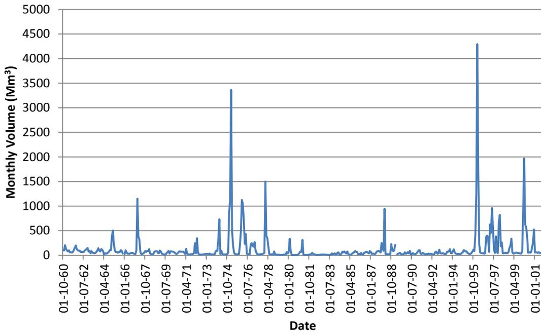
**Figure 3.15: Monthly Stream Flow Hydrograph at C2H018**
