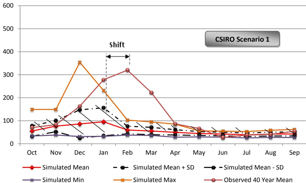
**Figure 6.26: Simulated Mean, Maximum, Minimum, One Standard Deviation & Historical Mean Monthly Stream Flows (CSIRO)**
