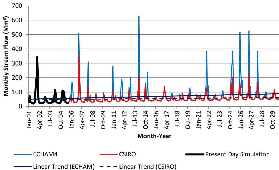
**Figure 6.36: Simulated Monthly Stream Flows for Overall Basin under Scenario 2**
