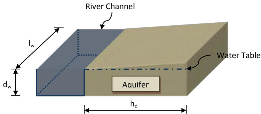
**Figure 4.6: Conceptual Representation of Groundwater in WEAP**
