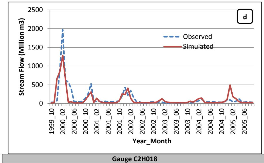
Figure 5.20: Simulation Results for Stream flow
