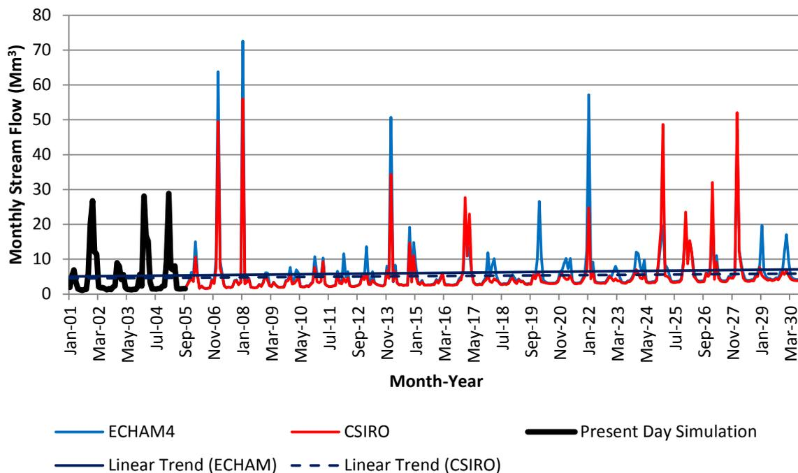
Figure 6.43: Simulated Stream Flows for Zone 3 under Scenario 3
