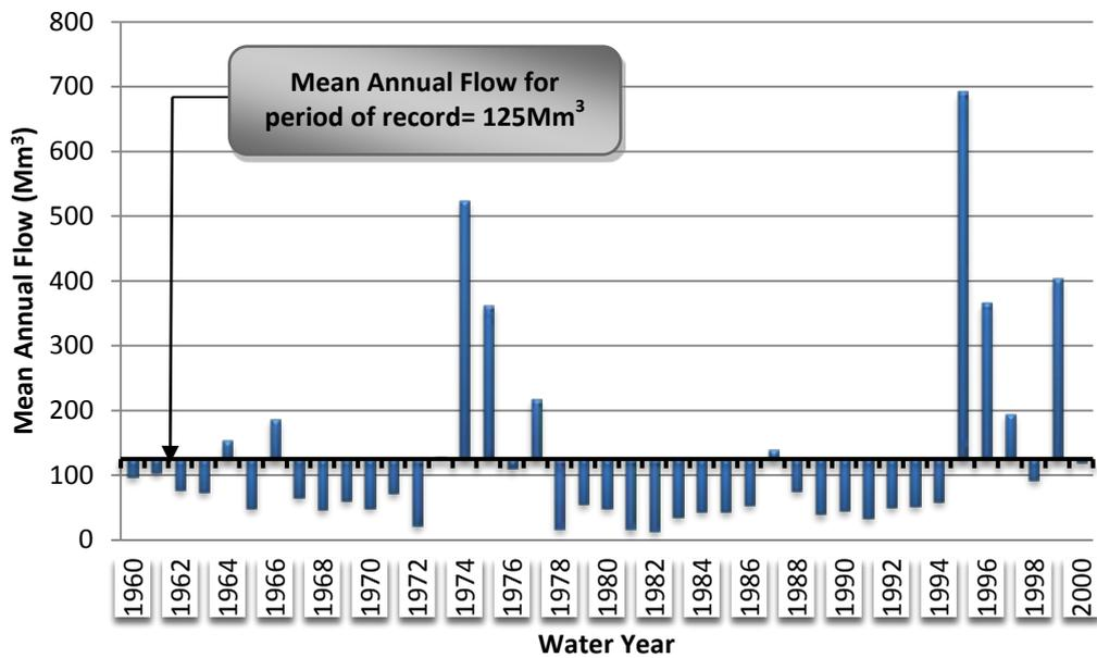
**Figure 3.16: Variation of Mean Annual Flow Volume around Mean Flow Volume at C2H018**
