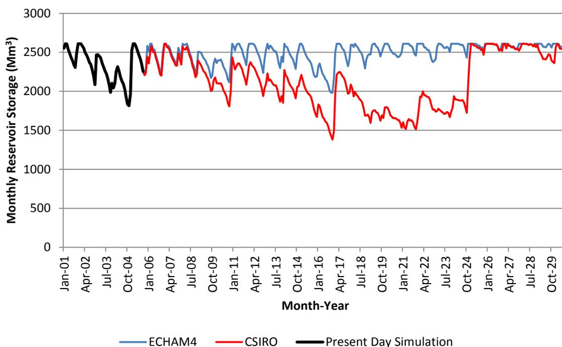
**Figure 6.49: Vaal Dam Simulated Reservoir Storage under Scenario 3**
